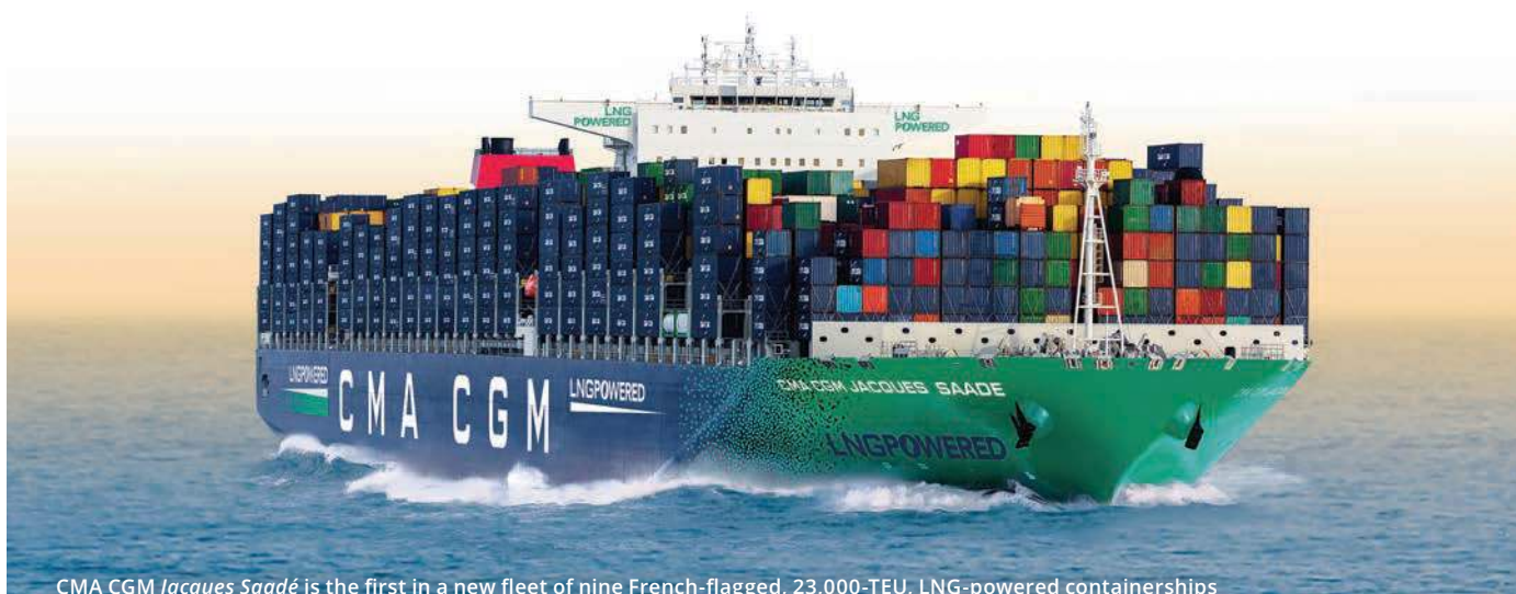
CMA CGM Jacques Saadé is the first in a new fleet of nine French-flagged, 23,000-TEU, LNG-powered containerships
