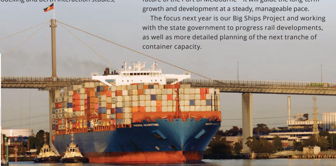
Maersk Skarstind at Port of Melbourne - close to 300m in length with a beam of 48.2m and a capacity of 9500 containers
